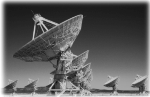
Image of the VLA near Socorro, New Mexico. The VLA consists of 27 individual radio telescopes (each of diameter 25 meters) that operate together to simulate one much larger telescope. Image taken by John M. Cannon.
